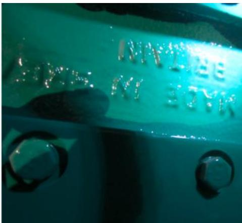
Counterfeit Cylinder Block marked "MADE IN GT. BRITAIN"
